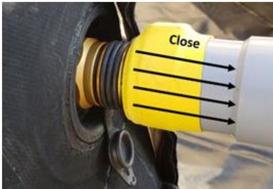
**Note:** The pressure relief valve opens at 4 PSI and self-resets (closes) at 3.5 PSI. This means that when the valve is opened, air will escape for some time until the lower pressure of 3.5 PSI is reached. The electric pump will not cause over inflation, but deployment with air bottles may cause damage, so ensure the pressure relief valves are clear of debris.
