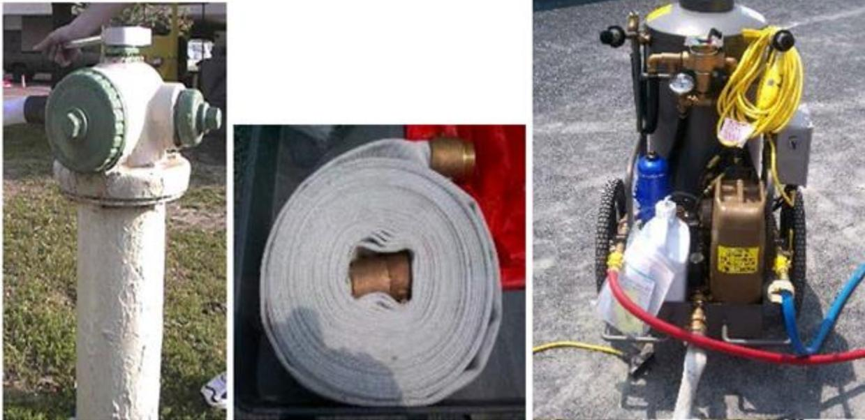
**Step 6.** Connect the red and blue water line camlocks to the water heater and the shelter as shown in [Figure A3.23](#). The red lines have decontaminant injected and flow toward the hot zone. The blue lines are for rinsing and flow toward the shelter's cold zone. **Note:** The red and blue colors do not indicate hot and cold water temperature.
