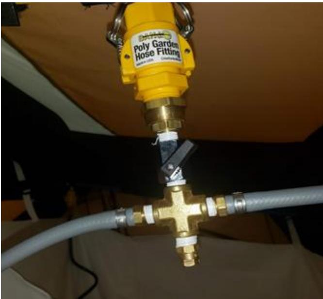
**Figure A3.48. Spray Wand Quick Connect.**
