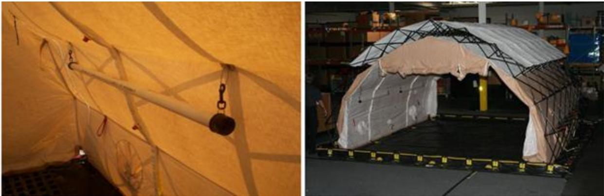
**Step 12.** Anchor the shelter. The shelter comes with an anchor kit that includes yellow lines and stakes (**Figure A3.16**).
