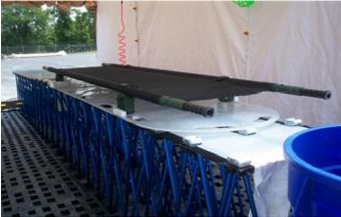
**Step 2.** Connect the Velcro in the middle of the conveyors and place the white safety stops on the two ends.
