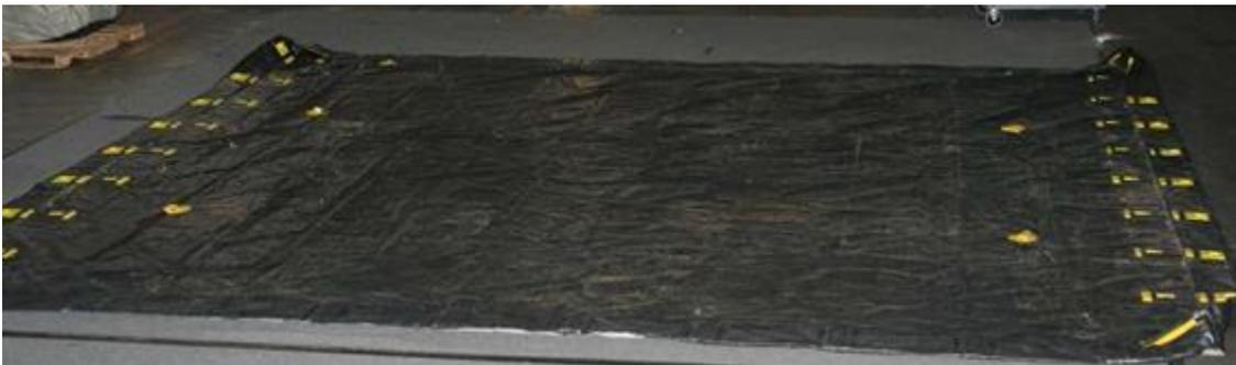
**Step 4.** Move the shelter bag to the center of the berm (**Figure A3.7.**). This step requires four people. Use the lifting straps located on the bag to move the shelter. Team members should lift high and avoid dragging the shelter. Assuming the shelter was packed correctly, the top should have yellow reflectors indicating the direction of the shelter throughput (**Figure A3.8.**).
